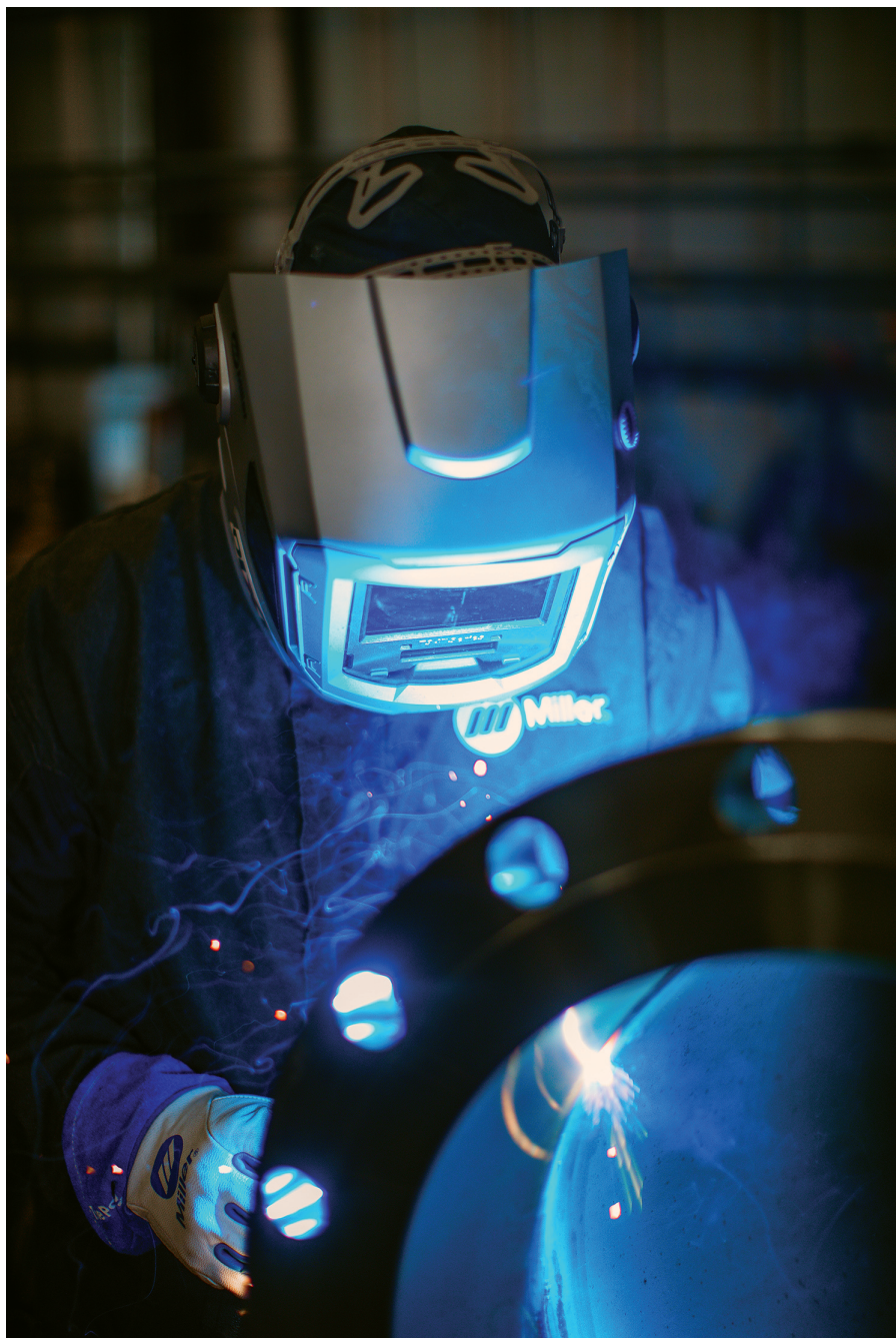
Fig. 1 — A switch to the Regulated Metal Deposition (RMD®) process eliminated back purge on stainless steel pipe welds, saving significant time and money.
