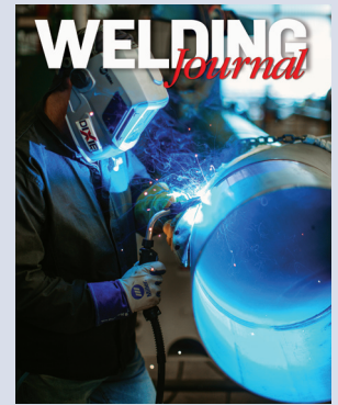
On the cover: A welder at Dixie Mechanical in Tuscaloosa, Ala., completes a pipe welding pass with the Miller® PipeWorx 400 multiprocess welding system. (Credit: Miller Electric Mfg. LLC.)
