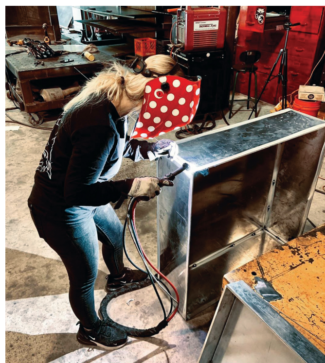
Fig. 1 — Stephanie Hoffman welds the beveled edges of the Statue of Liberty base. (Photo courtesy of Hoffman's Instagram @underground_metal_works .)
